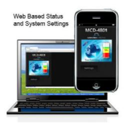
The MCD-4801 web interface can be accessed by any connected browser. Screens show battery life, data usage, wireless security settings, MAC address filtering, SMS messaging screens, and many other parameters.
