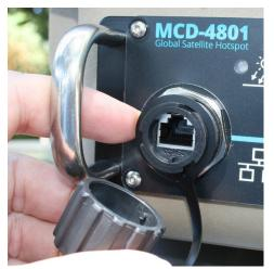
Both Ethernet LAN ports (RJ-45s) are available for hardwire connections. When not in use, it is capped to waterproof the case. Waterproof Ethernet connectors are also available. Please note the stainless steel bumpers to help protect the front panel from impacts.
