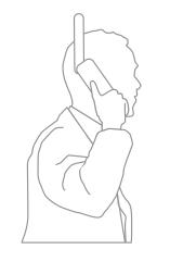
Stand outside with a clear view of the sky with the phone antenna pointing upwards. There must be a clear line of sight between the phone's antenna and the satellite.
