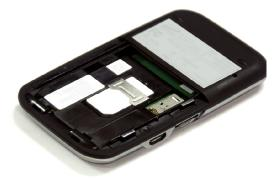
8 Insert the battery, lining up the contact points as shown, and then replace the door.
