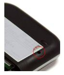
Insert a paper clip into the hole and hold the button down for five (5) seconds until the LED goes off.
