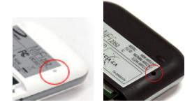
Insert a paperclip into the hole and hold the button down for 5 seconds until the LED goes off.
