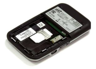
8 Now, insert the battery, lining up the contact points as shown and replace the door on the device.
