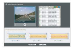
4 Move the control bar up/down to adjust the sensitivity range. If the range is wide, it is less sensitive, and if the range is narrow, it is more sensitive.
