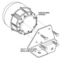
Secure the Howler siren speakers to the mounting brackets using the supplied sheet metal screws. Mount the speaker so the screened vent holes are facing down toward the road after mounting.
