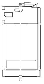
Figure 2 Storing the Antenna
