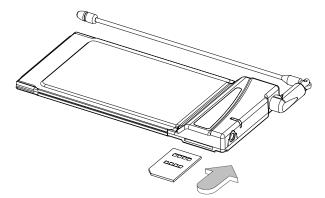
Figure 4 Inserting the SIM Card
