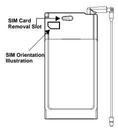
Figure 5 Removing the SIM Card
