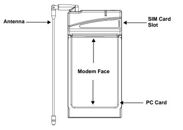
Figure 1 Modem Components
