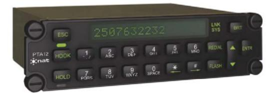
Using the full-function panel mounted dialer, FLIGHTDECK puts a phone in the cockpit. Perfect for any type of fixed-wing aircraft or helicopter, FLIGHTDECK can be connected to the aircraft's intercom system so that the phone can be used by a single crew member or shared by all intercom stations.
