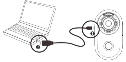
B) Connect another end of the computer data line to the USB port of the computer.
