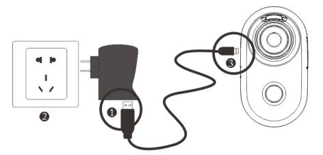
B) Plug the power adapter in the power socket.
